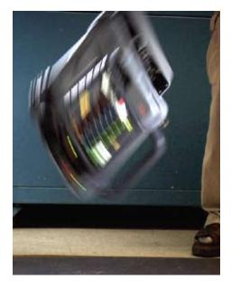
While Philips® drops the MRx® on all faces onto a steel surface at 30 inches with a carry case®, we drop the LIFEPAK 15 monitor/defibrillator onto a steel plate on all six sides from 30 inches WITHOUT a carry case.
