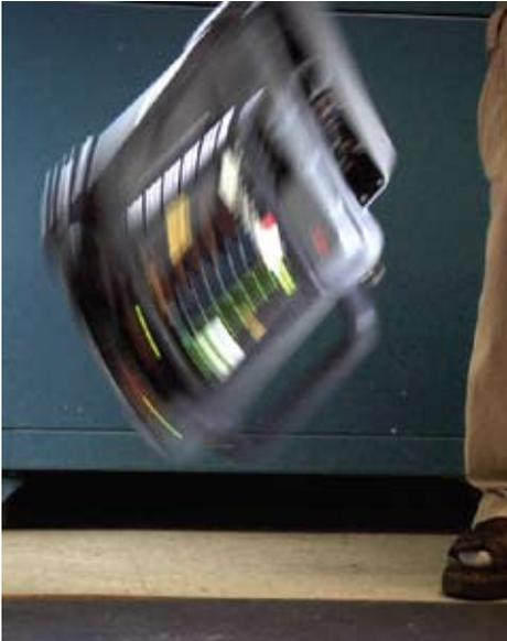
While Philips® drops the MRx® on all faces onto a steel surface at 30 inches with a carry case<sup>3</sup>, we drop the LIFEPAK 15 monitor/defibrillator onto a steel plate on all six sides from 30 inches **WITHOUT** a carry case.
